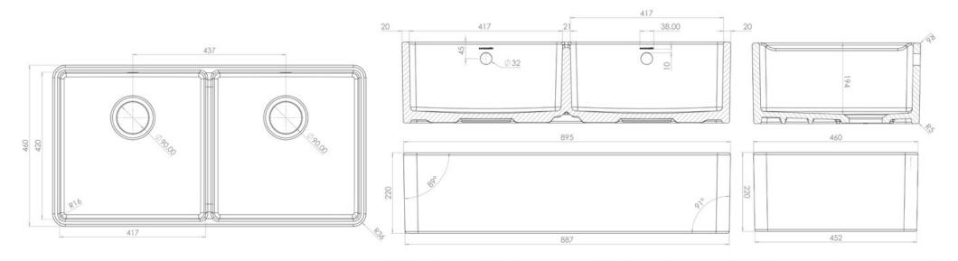
NB. Due to manufacturing processes this sink may have a +/- 4mm tolerance on the measurements
