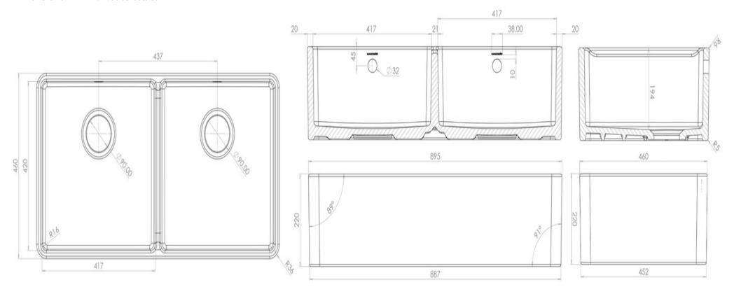
NB. Due to manufacturing processes this sink may have a +/- 4mm tolerance on the measurements
